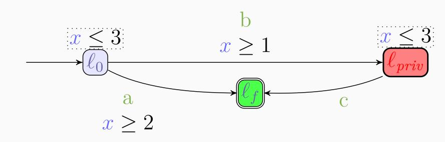
(timed opacity) The system is **opaque w.r.t.**  $\ell_{priv}$  on the way to  $\ell_f$ Definition for a duration d if there exist two runs from  $\ell_0$  to  $\ell_f$  of duration d
